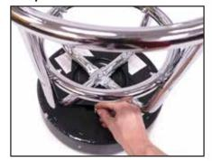
Turn assembled frame upside down and place on top of upside down pad. With swivel plates offset to allow access to the remaining bolts holes, insert the 4 brass bolts and tighten with Phillips screw driver.
