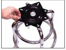
Offset the top swivel plate from the bottom plate to gain access to the bottom bolt holes and align with holes in the frame legs. Insert the 4 medium bolts and secure with the 4 remaining nuts. Tighten with Phillips screw driver.
